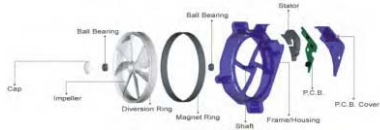
AC FAN Dimension : 120mm-254mm Thickness : 38mm-89mm Voltage: 110V-230V
