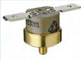
Termostatos 1/2" 40-180(195)°C, 230Vac-16(6)A
