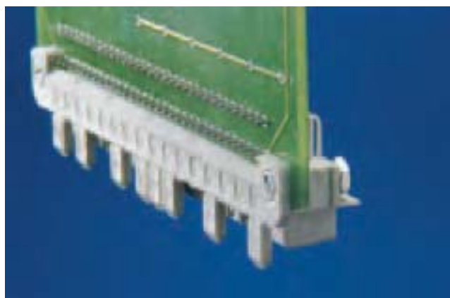
When coding the plug-in module, the coding strip M is always used. The M strips' coding tabs are identified with the letters A, B, C, . . . , P.
