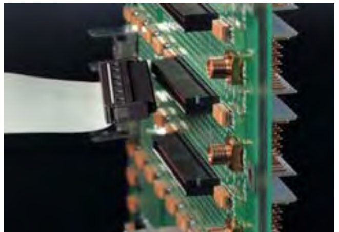
Rear I/O pressfit connectors on backplanes
