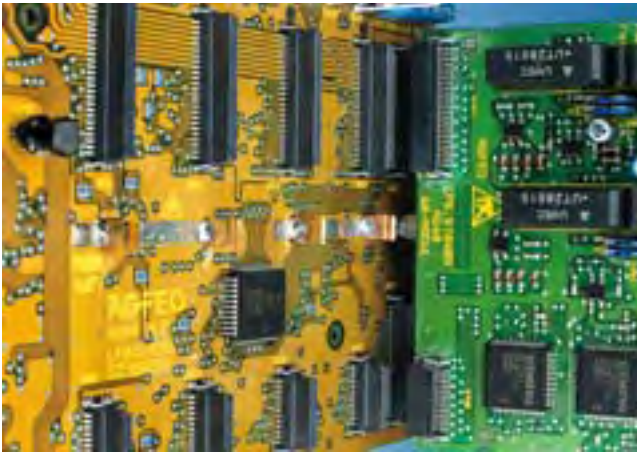
Motherboard to daughter card in an ISDN equipment
