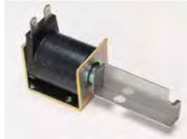
"C" Frame solenoid with integral mounting bracket, overmolded coil, special armature attachment, plunger stop and locking feature
