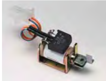
"C" Frame solenoid with special plunger end for optical sensing, and built-in full wave bridge rectifier for use with AC voltage
