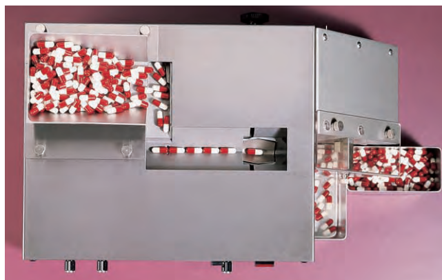
▲ Top view of balance shows automatic feed, individual weight readings, product removal and sorting.
