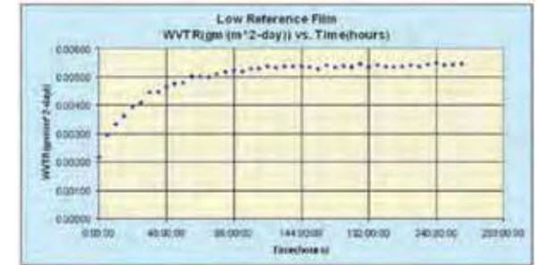
Actual data from test performed on AQUATRAN low reference film
