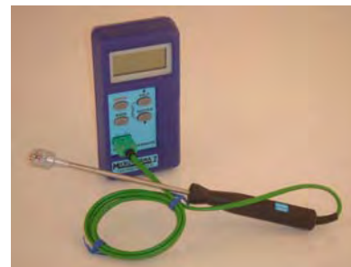
Thermometer and s/s band surface probe to check jaw temperatures.
