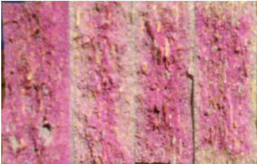
Figure 3 Carbonation of Viroc CBPB after 2 month exposure (from left to right: Free CO 2 →normal air→outdoor protected→weathering exposure)
