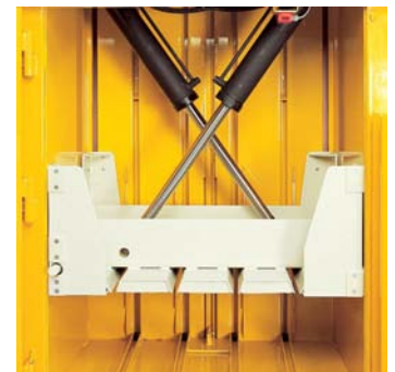
The scissor cylinders ensure stable compression and a low overall height.
