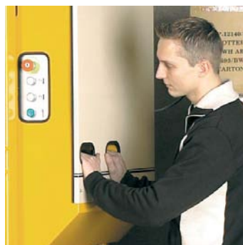
The bale is ejected by a safe two-hand operation.
